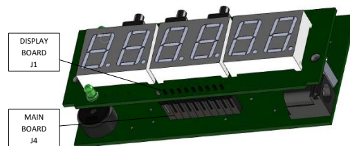
• Figure 11: Main and Display board Interface connector mounting
